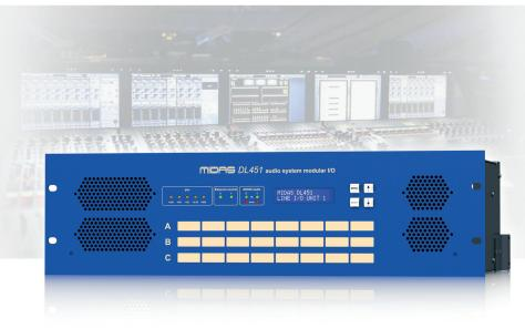
DL451 is a 3U 19" modular configurable rack mount I/O unit with provision for 3 DL4 Series interface cards and up to 24 audio inputs and 24 audio outputs. With two AES50 network ports and two Ethernet control ports providing dual redundancy, plus a MIDI Interface (In, Out, Thru), the DL451 is the ideal partner to all MIDAS Pro Series digital consoles, enabling a digital snake connection from Front of House to
